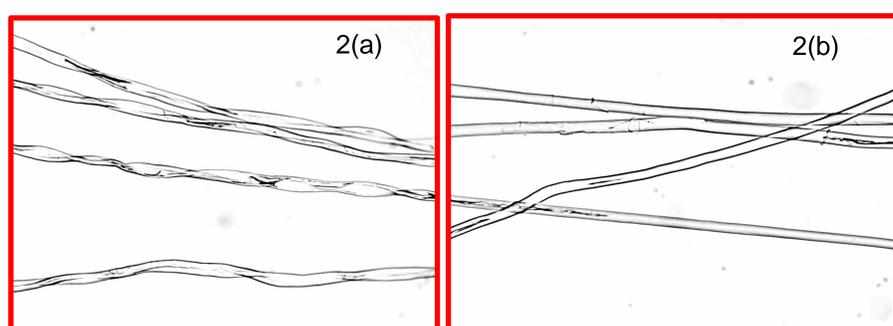
Figures 2(a) – (b): Optical microscopic images (x10) of scoured (a) and amino acid treated (b) cotton fibres
