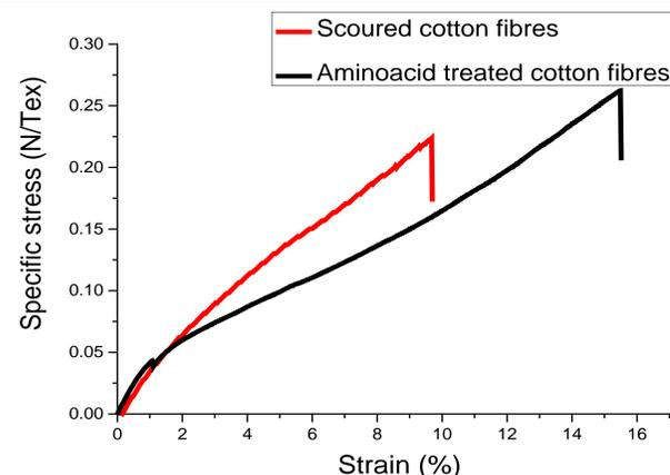
Figure 4: Specific stress- strain curve of scoured and amino acid treated cotton fibres
