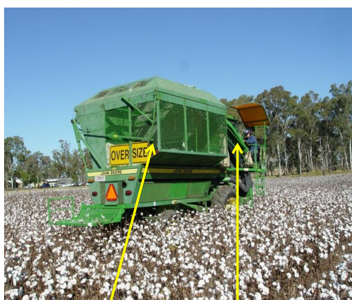
2010 internal weigh bin & external sampling shoot installed
