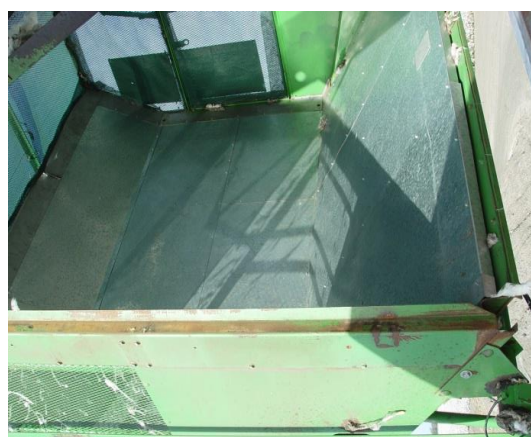
2013 internal bin removed with weigh cells added under a false floor
