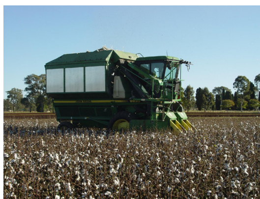
2013 internal bin removed with weigh cells added under a false floor
